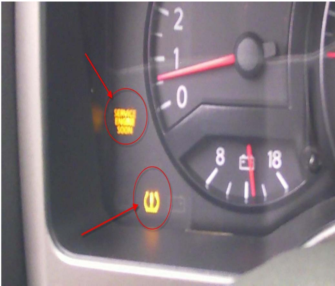
The top light is Service Engine Soon and bottom light is tire pressure monitor
